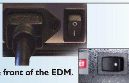
If it does not start up, toggle this switch located on the front of the EDM.
