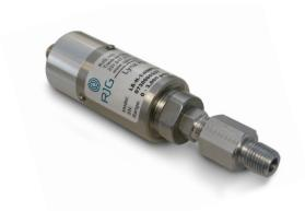
The Lynx™ 3,000/5,000 psi Hydraulic Pressure Sensor LS-H-1/4NPT-3K/5K is installed on the hydraulic system of injection molding machines in order to provide the eDART® or CoPilot® System with injection and back pressure data.
